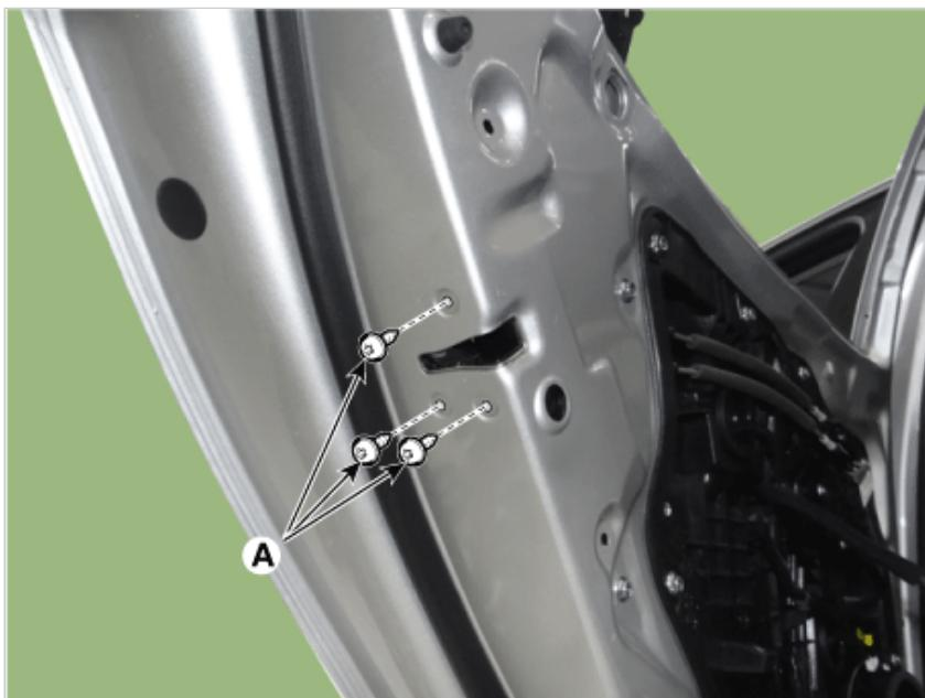
8. Remove the rear door module (A) after loosening the mounting bolts.
